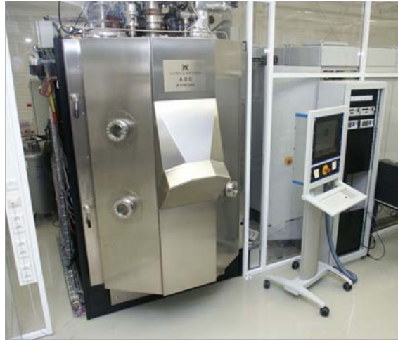
Figure 1.3: The Advanced Development Coater at FOM developed based on thin film process data described in this thesis.
