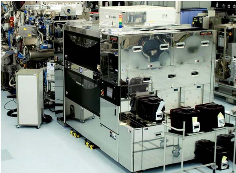
Figure 2.20: One of the proof-of-principle EUVL-exposure set-ups: Alpha Demo Tool (courtesy ASML).
